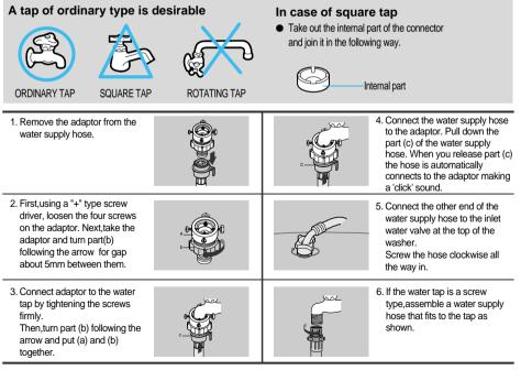
Note : The appliance is to be connected to the water mains using new hose-sets and that old hose-sets should not be used.
